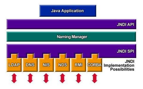
Figure 2: JNDI API and Service Provider Interface (SPI) [source: Oracle]
