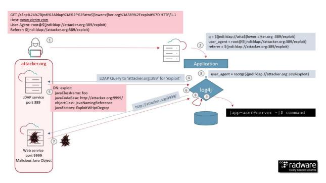
Figure 3: Remote command exection attack leveraging Log4Shell vulnerability [source: Radware]
